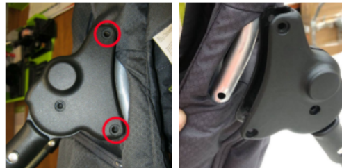
Bolt and washer missing
