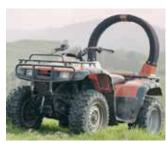
The ATV Lifeguard and Quadbar models referenced in the standard are as at 6 April 2019. However, the standard supports quad bike and aftermarket OPD manufacturers to develop designs for innovative OPDs to protect operators as long as it offers the same or better level of protection as the ATV Lifeguard or Quadbar.
