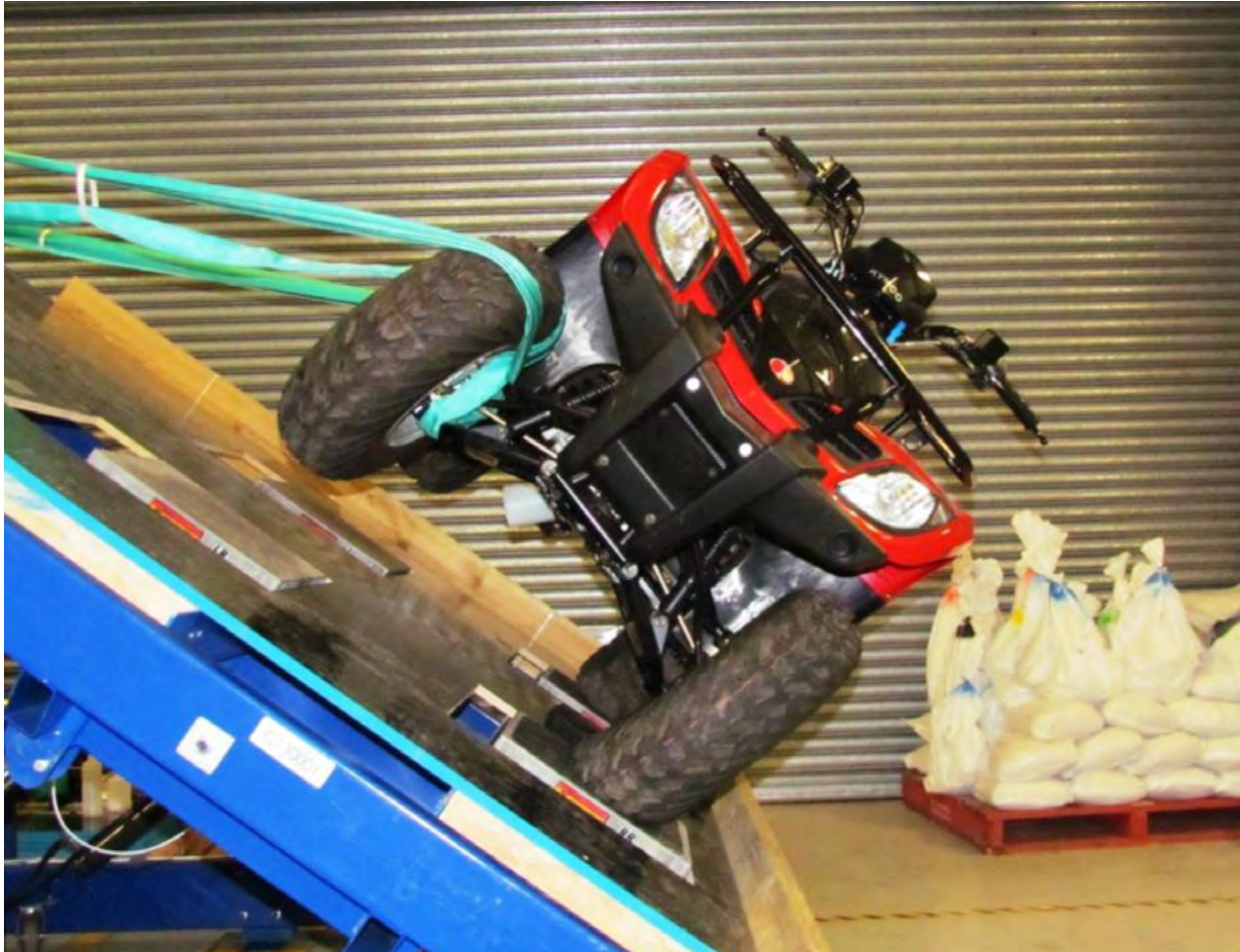
Figure 14: Typical tilt table quad bike lateral roll test 133
